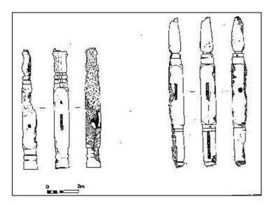
Figure 32: Measured drawings of two small turned posts, recovered from the unidentified wreck off Green Cape. They may belong to a fence or rail aboard the vessel. (Drawn by Tim Smith)
