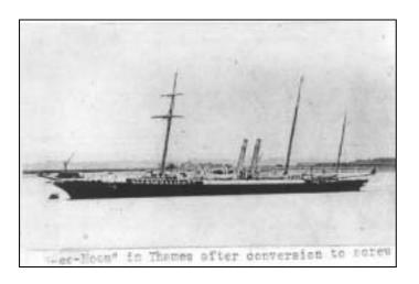
Figure 7: ss Ly-ee-Moon after conversion from paddle steamer to screw steamer. Courtesy: Mitchell Library, State Library of NSW.
