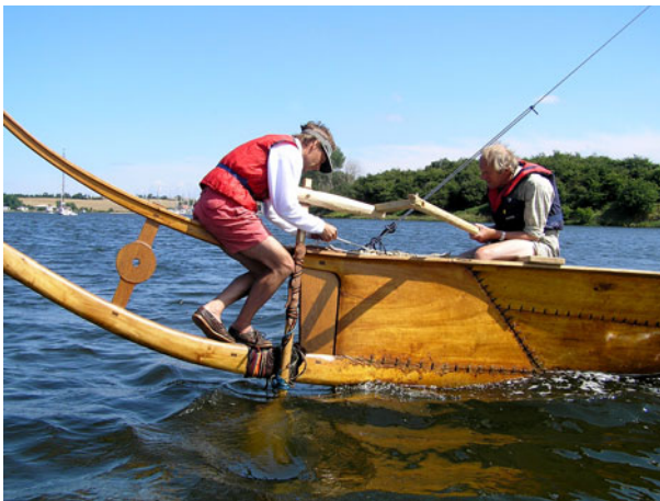
Fig. 25 Adjusting the forward steering oar. This shows the relative ease with which an agile crew member can climb the “horns” of the Tilia . (Photo: Knut Valbjørn)
