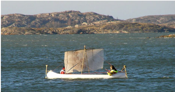
Fig. 9 The canoe in winds of 12–14 m/s. Notice the tilt of the yard towards the fore end of the vessel. (Photo: Vivian Leke)
