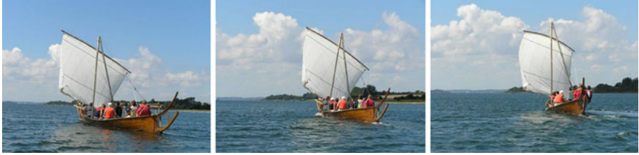
Fig. 32 Outside the gap on day 1. A gust hits the boat in picture three of this sequence. Notice the bubbles in the water caused by the turbulence around the steering oars which can be used to detect leeway. (Photos: Knut Valbjørn)
