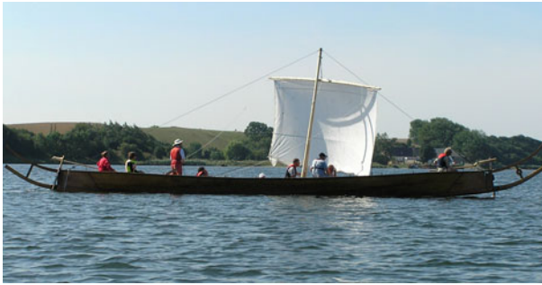
Fig. 26 Tilia on the second day of the sail trials in the light wind of Dyvig harbour. Notice the forward rake of the mast which is adjusted through lengthening or shortening the aft- and forestays. (Photo: Knut Valbjørn)
