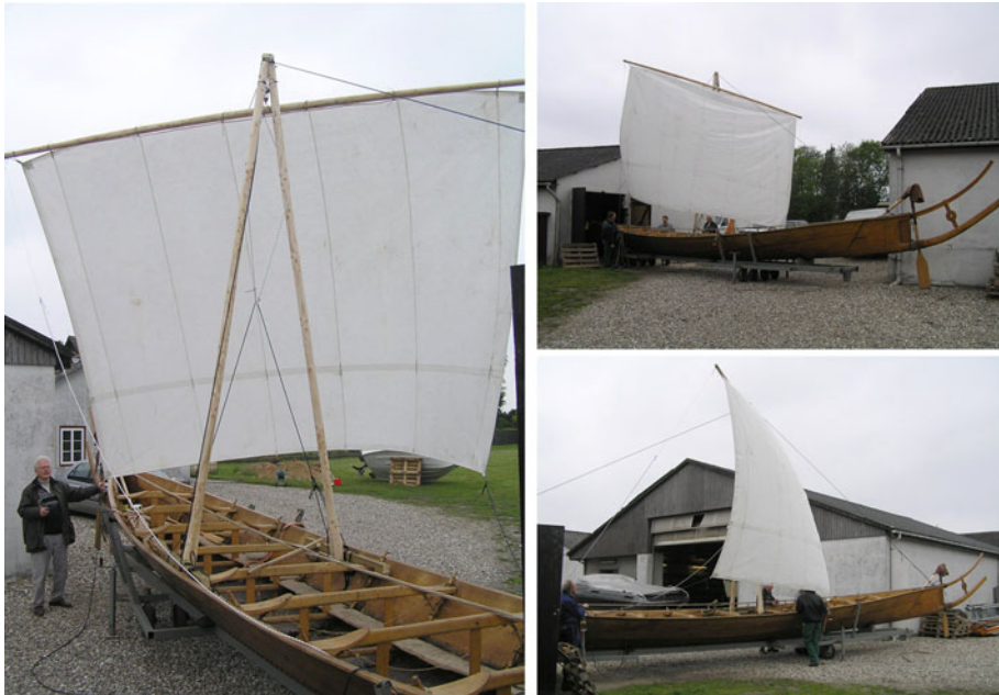
Fig. 22 Dry sailing the Tilia in May 2006. Here the full size of the sail can be appreciated. The reefing system can be seen as a lateral line across the lower end of the sail. (Photos: Boel Bengtsson)
