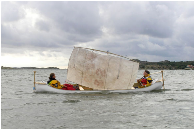
Fig. 10 Trials using the earlier and lower rig with the yard tilting towards the aft of the vessel. (Photo: Britt Bengtsson)
