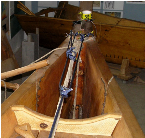
Fig. 19 The white trussing rope and the blue forestay are both attached to the same four integral cleats that are located at each end of the Tilia . (Photo: Boel Bengtsson)
